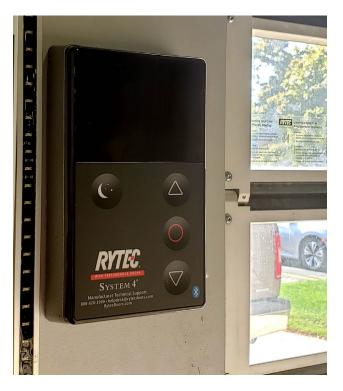
The BTA4 (Bluetooth Access) Controller – when connected to the Rytec System 4<sup>®</sup> - enhances the operation and aesthetics of our high-speed, high-performance doors. It provides a new wave of technology and accessibility that is in great demand. The BTA4 will allow Bluetooth access and control via iPhone or Android smart phones for service, programming and updating. BTA4 now makes it even easier to maintain door functionality.
