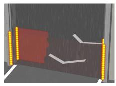
Recognizes when weather elements (rain/ snow/ice) block beams for prolonged period and closes door slowly. Minimizes door open time during these events as long as all other safeties are clear.
