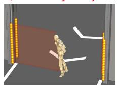
Reduced door opening/closing speed if beams are blocked, or abnormal traffic patterns or unusual doorway presence is detected.
