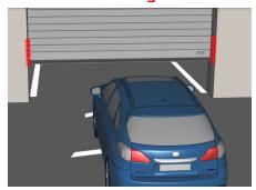
Cascading red in direction of movement when door is opening or closing.
